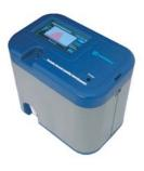
aerosol sampling applications. It provides the numberweighted diameter distribution of aerosols over the entire submicrometer range (10-1000 nm) in one scan. The unit Uses a non-radioactive bipolar aerosol charger to allow easy access to sampling sites with tight safety regulations. its bipolar charger significantly reduces measurement uncertainty of larger particles in the submicrometer range
