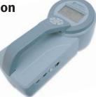
this advanced technology, users can implement nano-sized particle research in occupation and working areas. The Model 3800 is appropriate as a screening tool to evaluate filter performance and gasket leakage. It is also an optimal tool to detect black carbons, such as soot and smog, which are normal constituents of exhaust contaminants from combustion.
