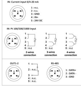
I/O connectors: Hirshmann EF12M5 (5 pin socket) + plug
