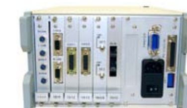
Model 1560 has 6 slots for modules
