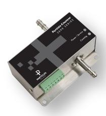
The Particles Plus 2501-4 Remote Particle Counter measures 0.5  $\mu$ m, 0.7  $\mu$ m, 1.0  $\mu$ m & 5.0  $\mu$ m with a flow rate of 0.1 CFM (2.83 LPM). Integration is easy into a real-time monitoring or building management system via Modbus RTU or ASCII. The 2501 models are the smallest remote particle counters in the market and have easy mounting options. The Particles Plus 2501-4 units comply with ISO 21501-4 and include a 2 year limited warranty.
