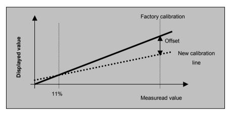
Factory calibration can be obtained by entering offset 0.0
